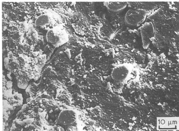
Figure 6 Failure cracks at the fibre-matrix interface and between the fibres.
